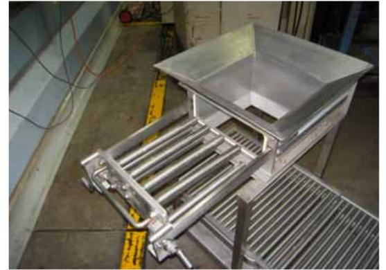
sugar production, grain production, bulk products, cereals manufacture and milk powder, MAGNATTACK™ GLOBAL supplies to some of Australia's leading food manufacturing companies. This self-cleaning magnet can be supplied worldwide including the USA. For more information on the self-cleaning magnet and other magnets please visit our website to view the full range of magnetic products and services.
